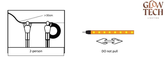
Do not allow the tape to sag or hang, as this can damage the electrical connections within it.
