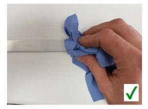
Ensure the tape is adhered to a clean metallic surface to dissipate heat. Do not Reposition once adhered.
