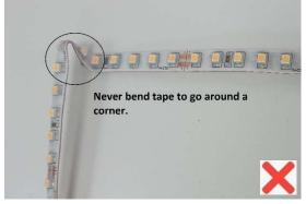
Never bend or twist the tape around corners as overheating and failure can result
