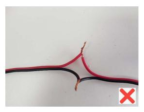
Ensure all connections are good, and of a Suitable IP rating for the application. Poor Connections can draw in moisture.
